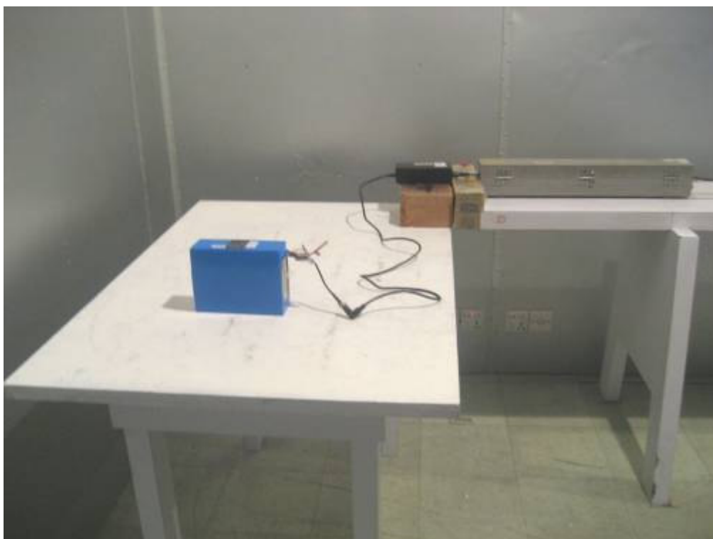
Figure 4 Disturbance power test set-up
