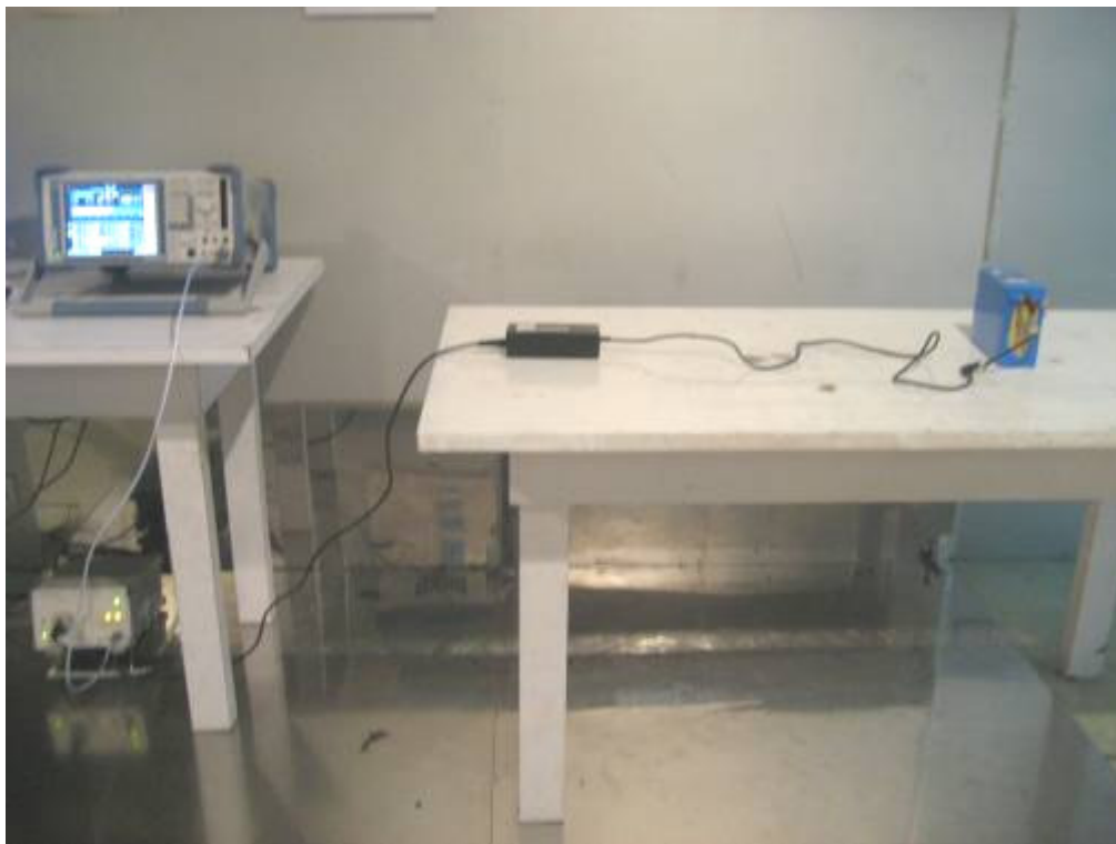
Figure 3 Conducted emission test set-up
